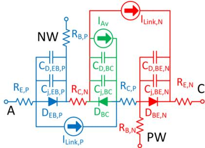
Fig. 1. Circuit representation of model. Components associated with the NPN and PNP are labeled with ‘N’ and ‘P,’ respectively. Components associated with the shared bases/collectors created by the NW/PW junction are labeled with ‘BC.’ The potential drop between the A and C terminals has three components: diodes drops, resistive drops across the conductivity modulated collector resistances, and ohmic drops across the emitter resistances.
