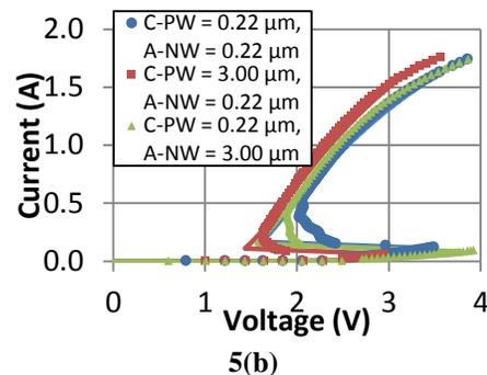
Fig. 5. Measured and simulated pulsed I-V characteristics of DTSCRs in a 130nm CMOS process. (a) Devices have varying anode to cathode spacing; geometric scalability is achieved by using measured  $\beta$  values and linearly extrapolated  $R_{C0}$ ,  $Q_{C0}$ , and  $\tau_R$  values. (b) Devices with varying well tap spacings.  $R_B$  is a non-linear function of well tap spacing.
