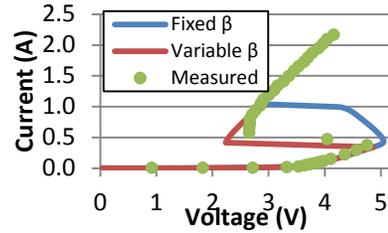
Fig. 3. Measured and simulated I-V curves for a DTSCR in 65nm CMOS. Using the measured  $\beta_{N0}$  of the 3-terminal NPN yields a poor fit where both transistors are active, i.e. the NDR region. The measurement data suggest  $R_{on} \approx 0$  near the holding point; this is attributed to non-uniform conduction across the device width [6], which existing models—[2-4] and this work—don’t replicate.
